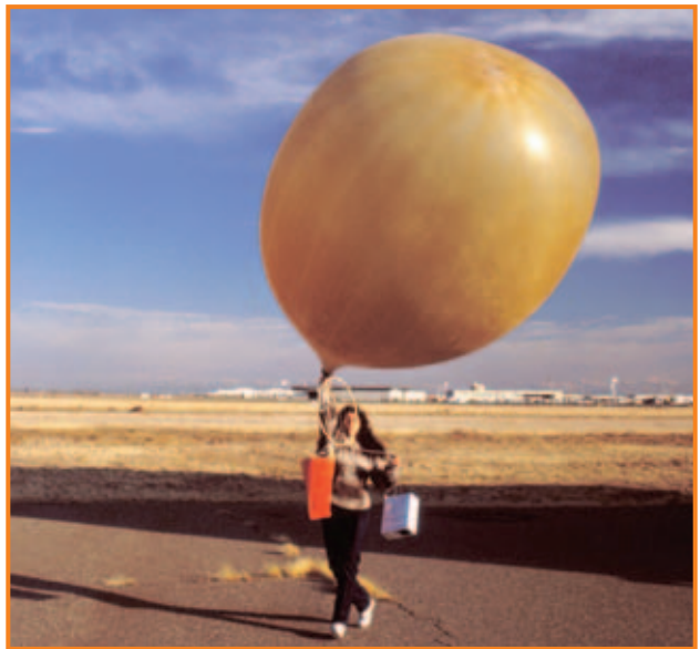
▲ Weather balloons carry instruments that measure temperature, air pressure, and humidity.
