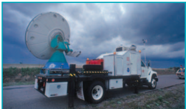
▲ Doppler radar detects the speed and direction of clouds and rain.
